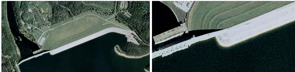
Figure 506.1: Dam satellite picture. Upstream (south facing) three dimensional slope at connection of the embankment and concrete gravity dam is evaluated for potential stability problem.
