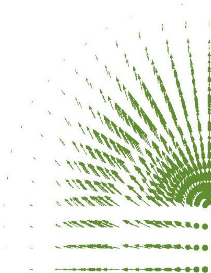
Figure 506.20: Plan view of a 3D undrained case, displacement vectors, lake and embankment at 680 ft, FS_{3D} = 2.00 .
