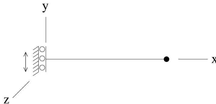
Figure 308.2: Finite element model for dynamic analysis
