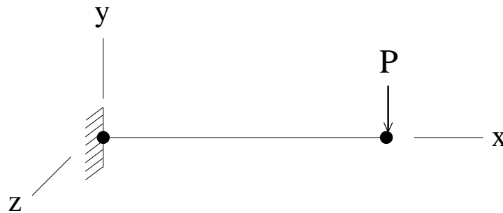
Figure 308.1: Finite element model for static analysis
