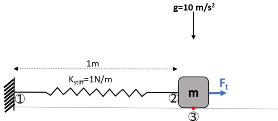
Figure 3.41: Illustration of frictional single degree of freedom problem
