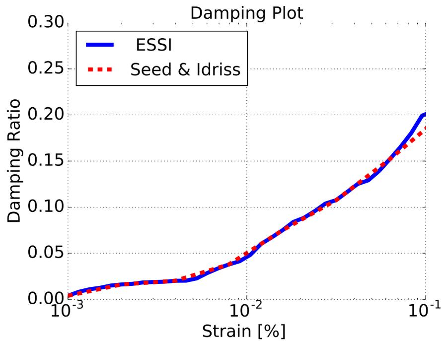
Figure 1.26: Damping Ratio Plot
