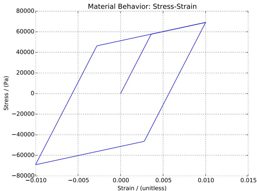
Figure 1.13: Kinematic Hardening Pure Shear Cyclic Loading.
