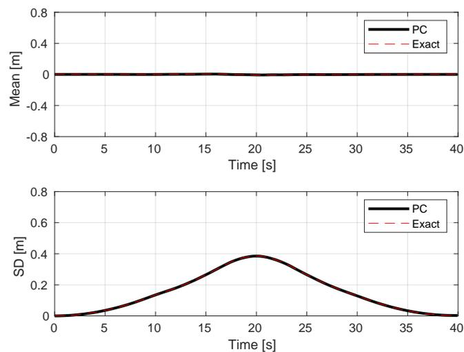
Figure 4.3: Verification of marginal statistics of random process motions.
