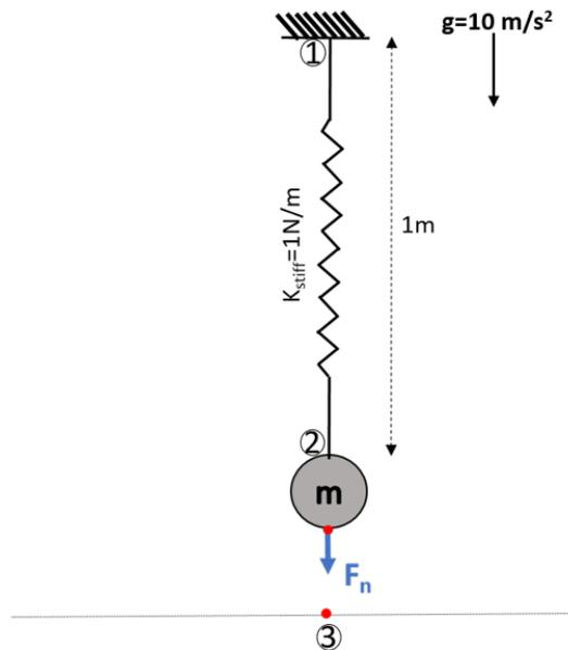
Figure 3.37: Illustration of one bar normal contact/interface dynamics
