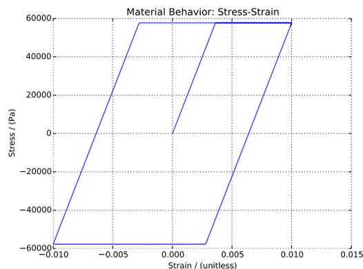
Figure 1.6: Perfectly Plastic Pure Shear Cyclic Loading.
