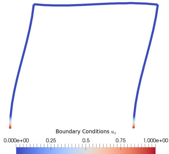
Figure 6.34: Boundary condition  $u_x$  for fiber beam pushover.
