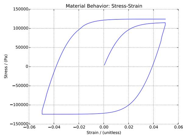
Figure 2.91: Results of No-Convergence-Check Pure Shear Cyclic Loading.
