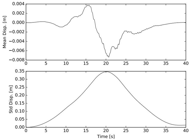
Figure 4.8: Probabilistic displacement response of ground surface.
