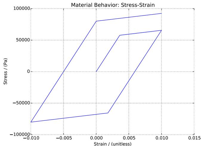
Figure 1.9: Isotropic Hardening Pure Shear Cyclic Loading.
