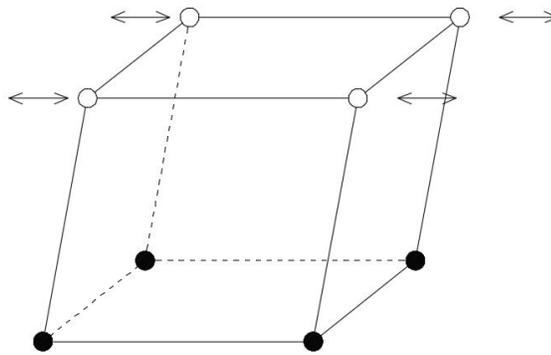
Figure 2.56: Perfectly Plastic Pure Shear Cyclic Loading.
