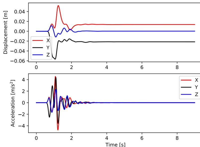
Figure 6.61: Time series response of 3C motion.
