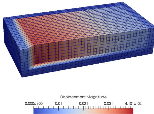
Figure 6.65: Simulation of 3D free field model under 3C seismic motion.
