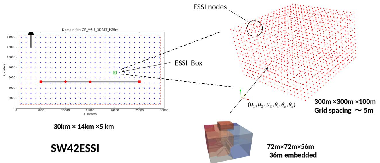
Figure 6.63: Illustration of transition from SW4 to Real-ESSI.
