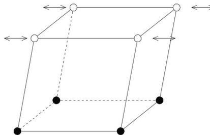
Figure 2.40: Perfectly Plastic Pure Shear Cyclic Loading.
