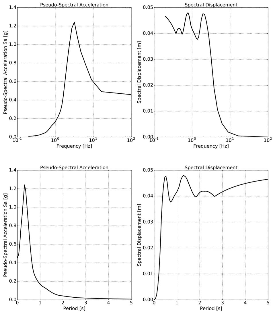
Figure 6.4: Simulation results: response spectrum at soil top.
