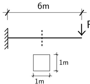
Figure 2.22: Problem description for cantilever beams.
