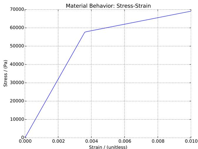
Figure 1.8: Isotropic Hardening Pure Shear Monotonic Loading
