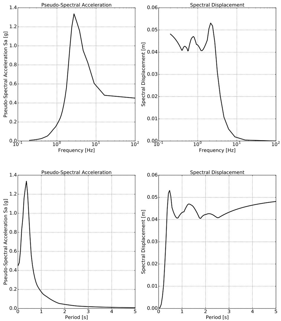
Figure 6.8: Simulation results: response spectrum at soil top.
