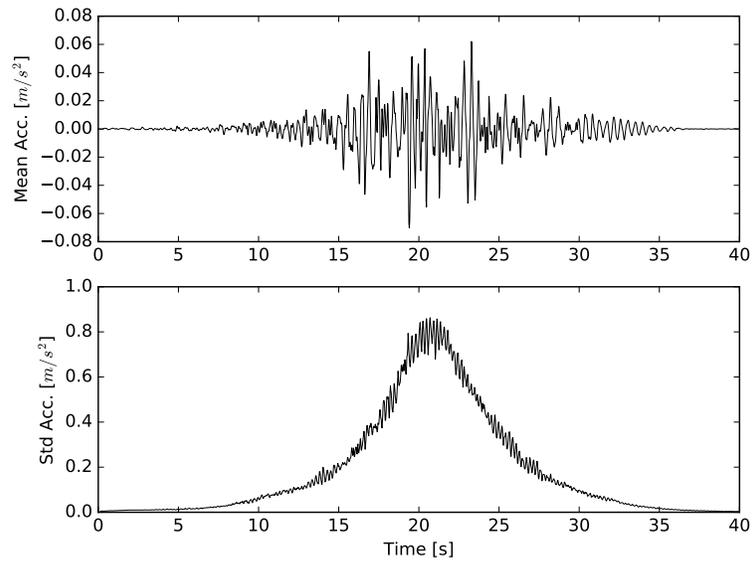
Figure 4.9: Probabilistic acceleration response of ground surface.
