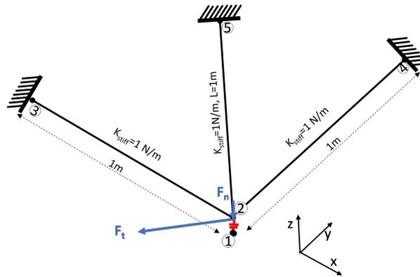
Figure 2.34: Illustration of 3-D Truss Problem with confinement loading in z-direction of 0.5N and then shear loading of 0.5N in x-y plane.
