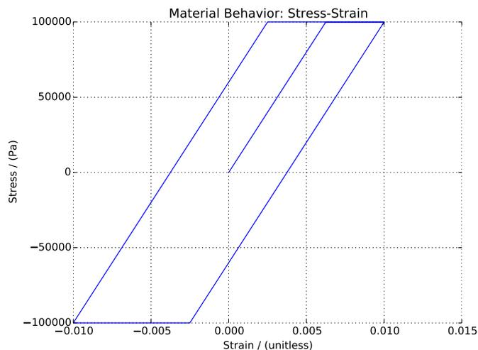
Figure 1.7: Perfectly Plastic Uniaxial Cyclic Loading
