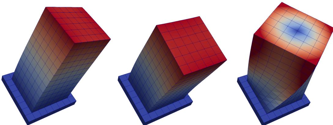
Figure 6.18: Eigen frequencies:  $f_1 = 3.47\text{Hz}$   $f_2 = 3.47\text{Hz}$   $f_3 = 6.88\text{Hz}$  (eigen mode 1 to 3 from left to right).
