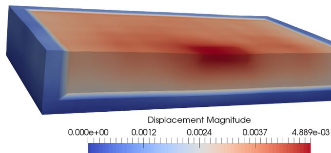
Figure 6.10: Soil foundation interaction results.
