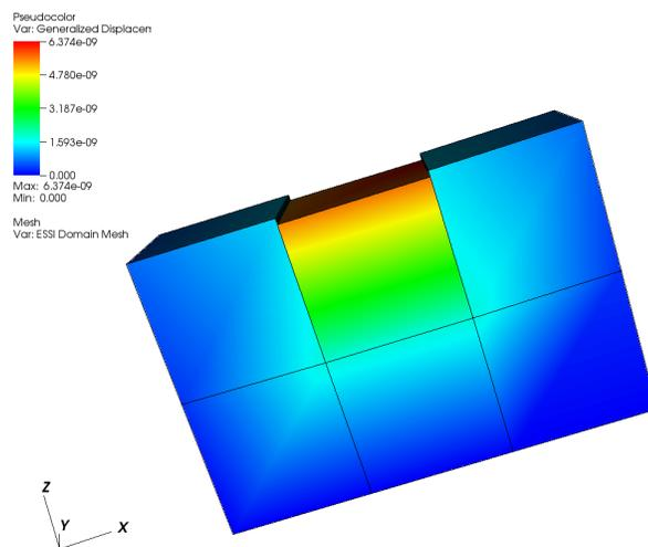
Figure 2.38: Generalized displacement magnitude visualization of normal loading.
