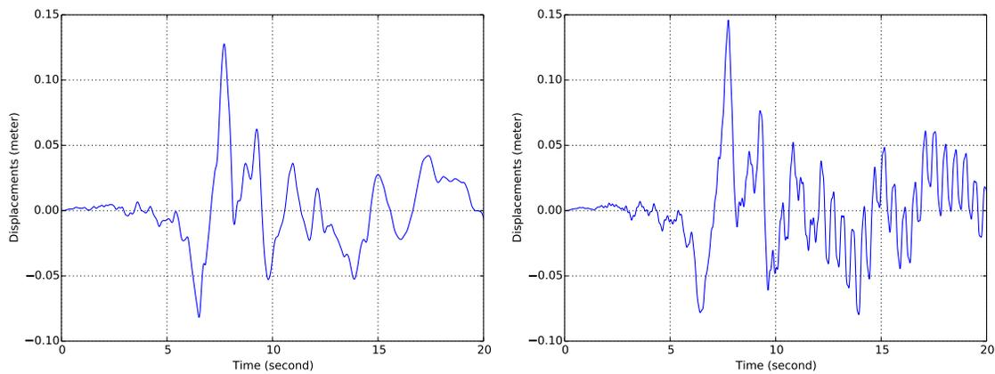
Figure 3.6: Input Motion (Left) And Output Motion (Right)
