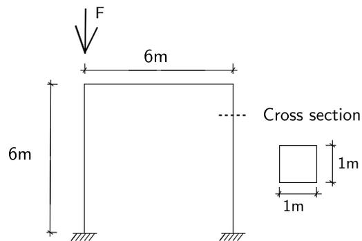
Figure 2.100: Elastic frame with *beam\_elastic* elements.
