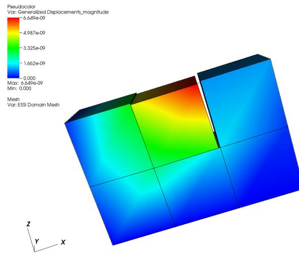
Figure 2.105: Generalized displacement magnitude visualization of tangential loading.
