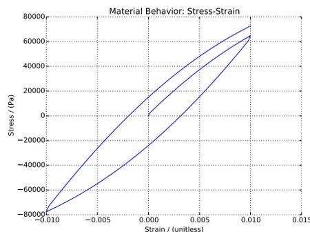
Figure 1.17: Drucker-Prager Armstrong-Frederick under Pure Shear Cyclic Loading.
