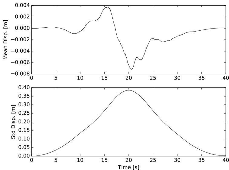
Figure 4.6: Probabilistic displacement response of ground surface.
