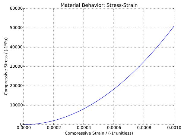
Figure 1.5: Results of Duncan-Chang Nonlinear Elastic Monotonic Loading
