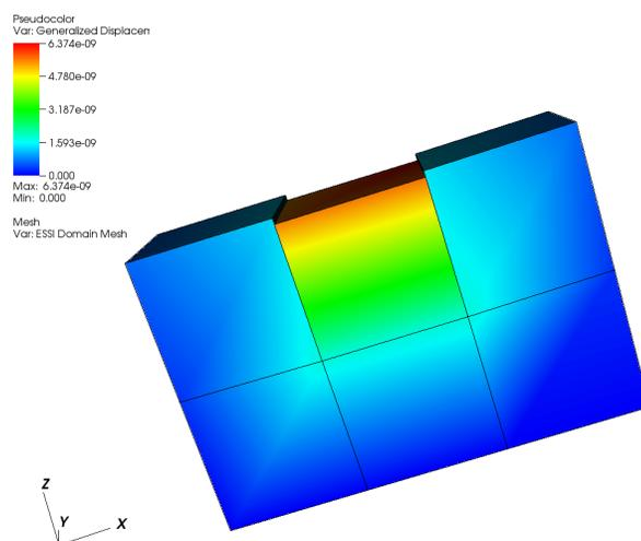
Figure 2.104: Generalized displacement magnitude visualization of normal loading.
