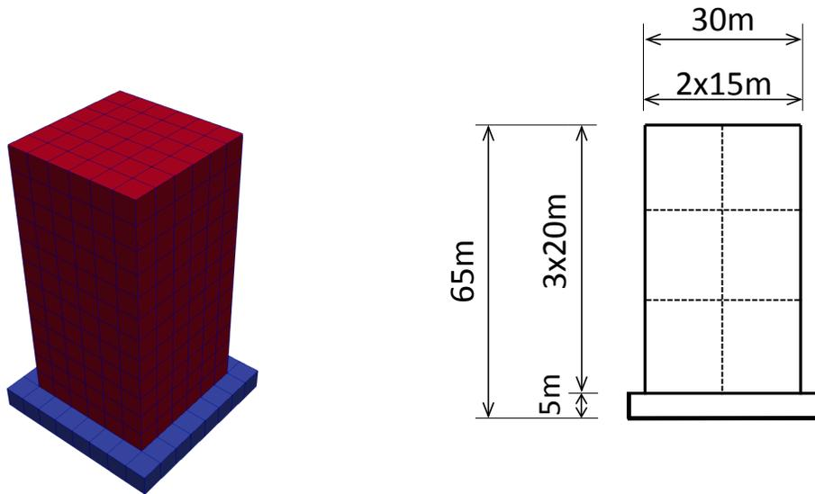
Figure 6.17: Structure on a fixed based simulation model.
