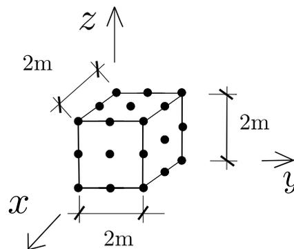
Figure 2.10: One element with surface load.
