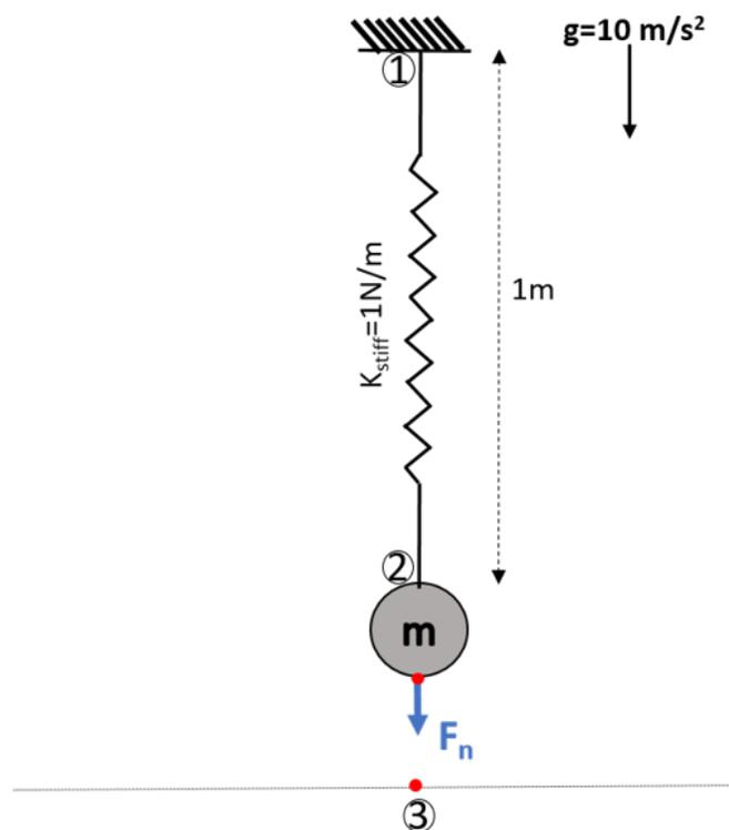
Figure 3.29: Illustration of one bar normal contact/interface dynamics.
