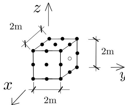
Figure 2.16: One variable Node Brick elements.
