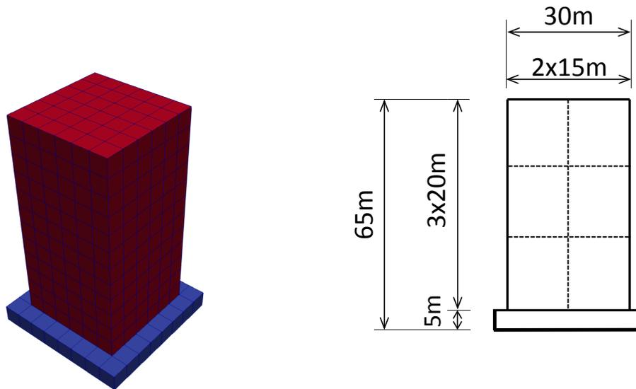
Figure 6.20: Simulation Model.
