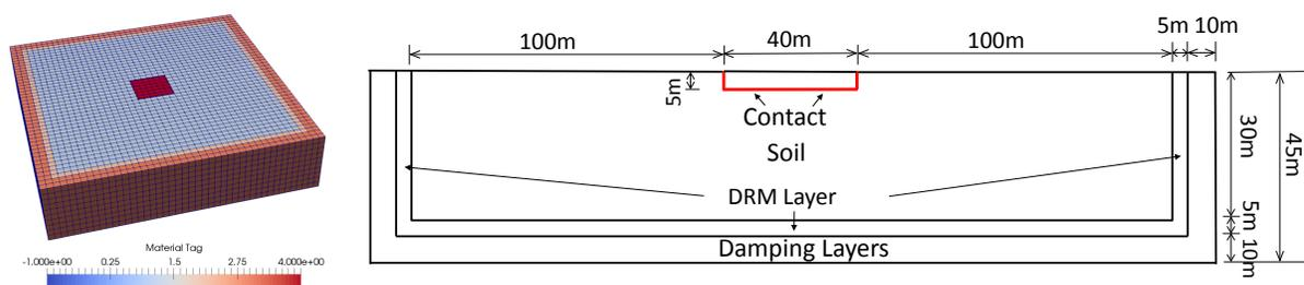
Figure 6.9: Simulation model.
