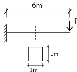
Figure 2.3: Problem description for cantilever beams.
