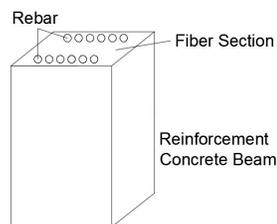
Figure 2.81: Diagram of the Beam with Fiber Section.
