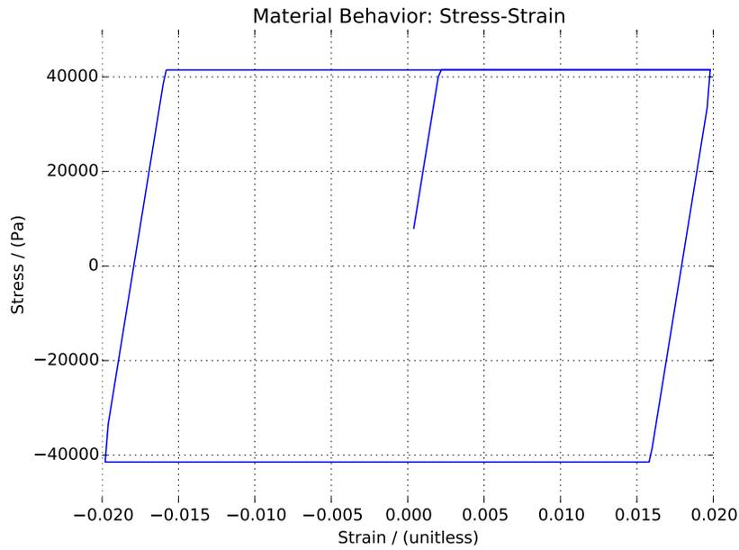
Figure 2.63: Results of Drucker Prager Yield Surface with Purely Deviatoric Plastic Flow under Pure Shear Cyclic Loading.
