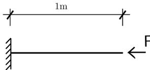
Figure 2.17: Problem description for a cantilever.
