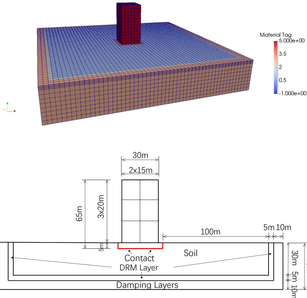
Figure 6.11: Simulation Model.
