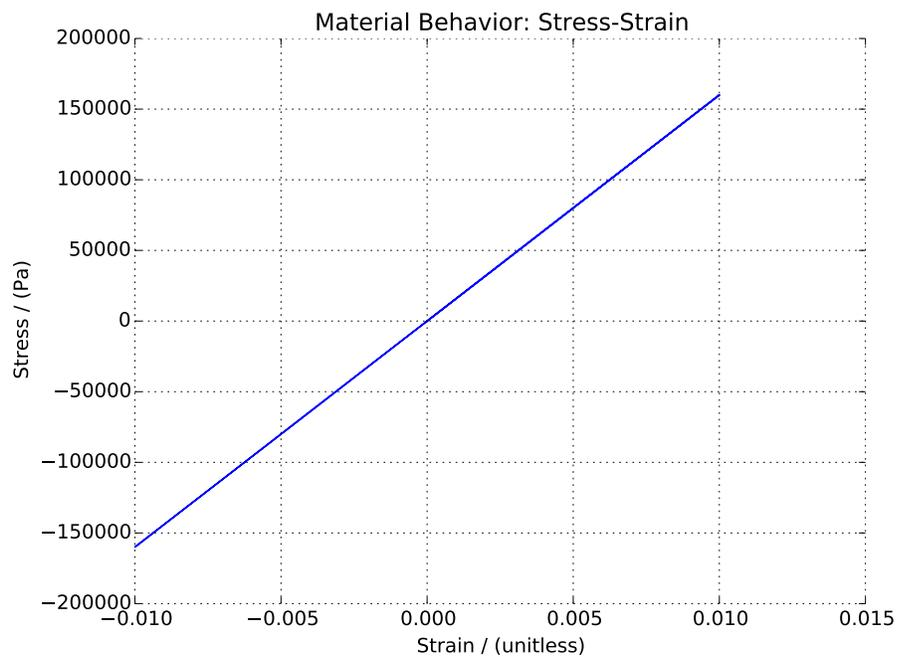
Figure 1.2: Linear Elastic Pure Shear Cyclic Loading.
