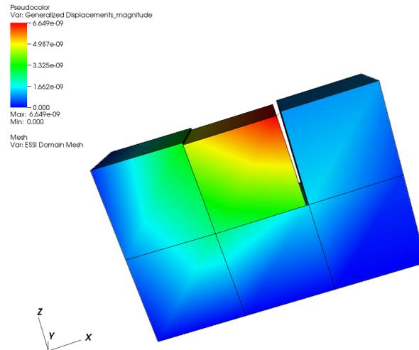
Figure 2.39: Generalized displacement magnitude visualization of tangential loading.
