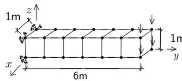
Figure 2.2: Six 8NodeBrick elements.
