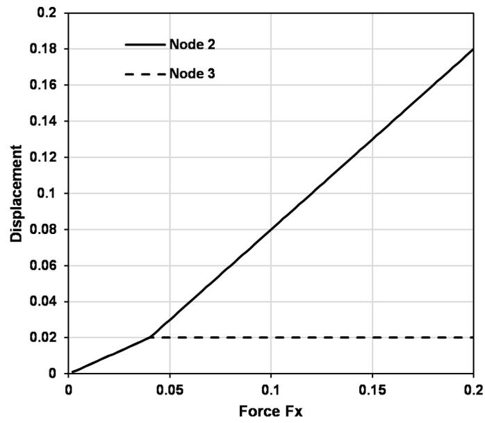
Figure 2.33: Displacement of Nodes 2 and 3 along y direction.
