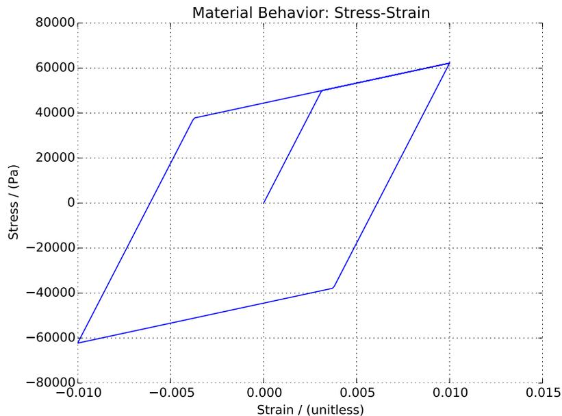
Figure 1.15: Kinematic Hardening Uniaxial Cyclic Loading
