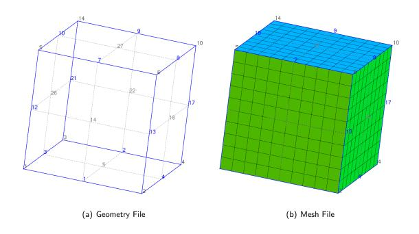
Figure 1.11: Gmsh geometry and mesh file for Example\_1
