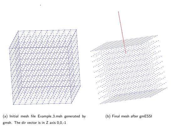
Figure 1.8: Example 3 Contact Problem. (b) shows the nodes and elements generated by gmESSI Translator.
