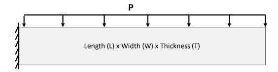
Figure 1.13: Illustration of the cantilever problem.
