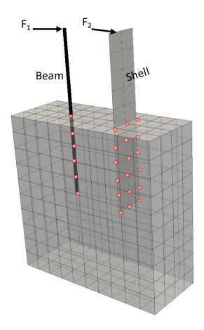
Figure 1.15: Illustration of the cantilever problem.
