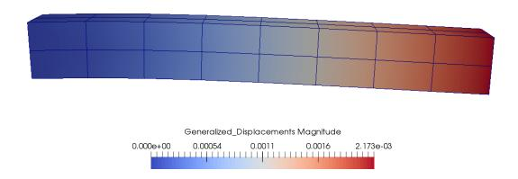
Figure 1.14: Illustration of the cantilever problem.
