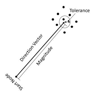
Figure 1.7: Pictorial representation of working of connect command.
