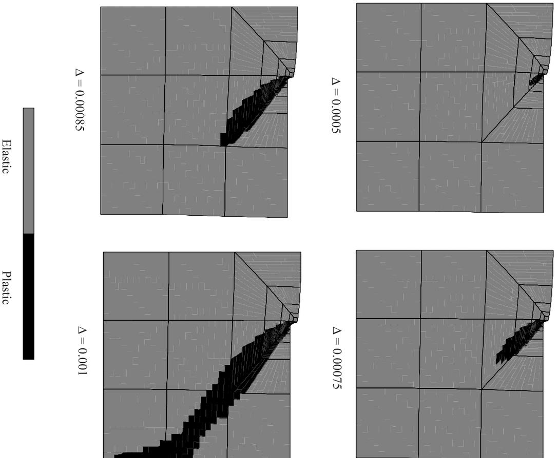
Figure 6: Progression of the localized plastic zone for  $p = 8$ .
