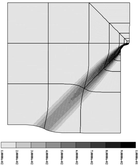
Figure 4: Equivalent strain  $\bar{\epsilon}$  for  $p = 8$ .
