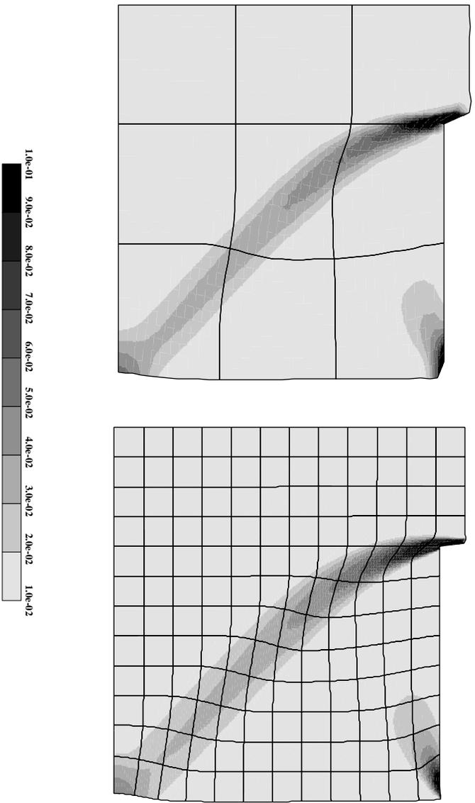
Figure 7: Equivalent strain  $\bar{\epsilon}$  for 3 by 3 mesh and 12 by 12 mesh,  $p = 8$ .
