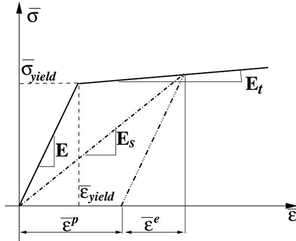
Figure 1: Elastic plastic effective stress effective strain bilinear model
