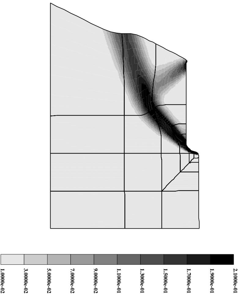
Figure 8: Equivalent strain  $\bar{\epsilon}$  for the slope stability problem,  $p = 8$ .
