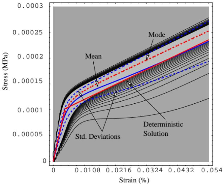
linear elastic – linear hardening elastic-plastic von Mises
