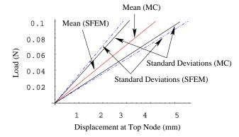
Mean and standard deviations of displacement at the top node, linear elastic material model, KL-dimension=2, order of PC=2.
