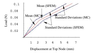
Mean and standard deviations of displacement at the top node, von Mises elastic-plastic linear hardening material model, KL-dimension=2, order of PC=2.
