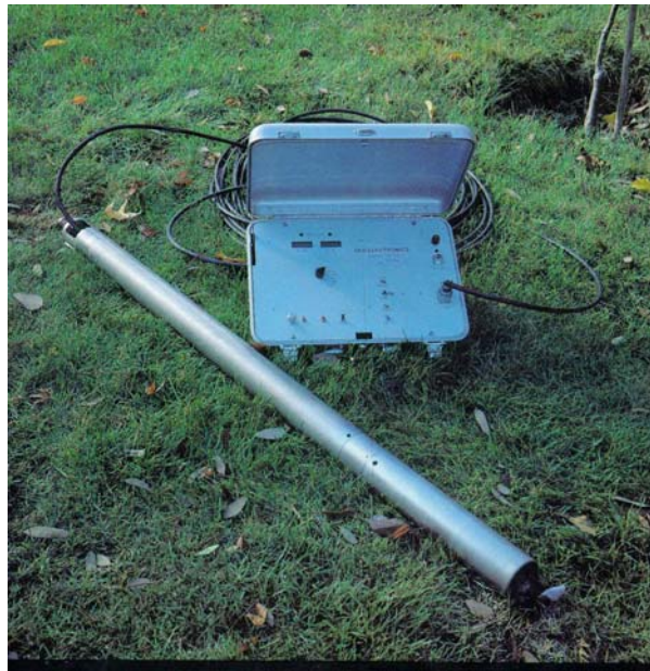
Figure 3.1 GEOELECTRONICS Electrical Formation Factor Probe with Control Unit and Cable
