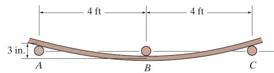
3. The beam is supported by a pin at  $A$ , a roller at  $B$ , and a post having a diameter of 50 mm at  $C$ . Determine the support reactions at  $A$ ,  $B$ , and  $C$ . The post and the beam are made of the same material having a modulus of elasticity  $E = 200$  GPa, and the beam has a moment of inertia  $I = 255(10^6)$  mm<sup>4</sup>.
